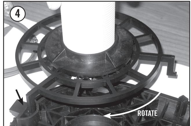
4) Re-installing the ERT carriage is accomplished by simply reversing steps 2 and 3. Insert one locking leg into the "D" shaped lock on the lid. Making sure the nib is aligned with the opening in the "D" shape, rotate the carriage until the legs are aligned with the secondary locks.
