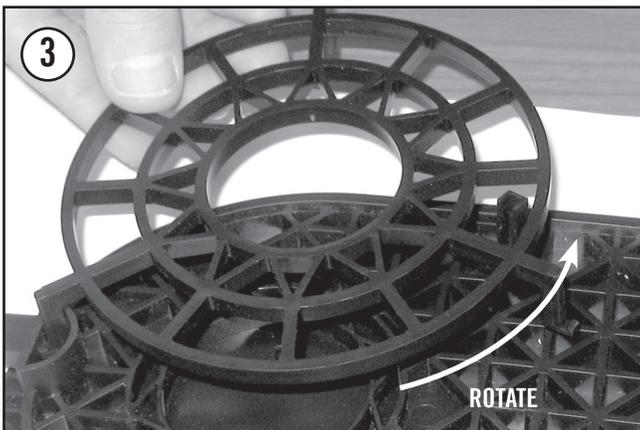
3) Keeping the carriage in a level position, rotate the entire assembly to unlock the third connecting leg. Gently pull upward.
